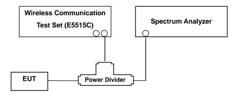
(Configuration of conducted Emission measurement)
