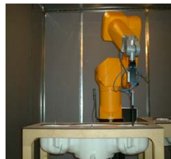
Figure 6.1 DASY4 Test System
