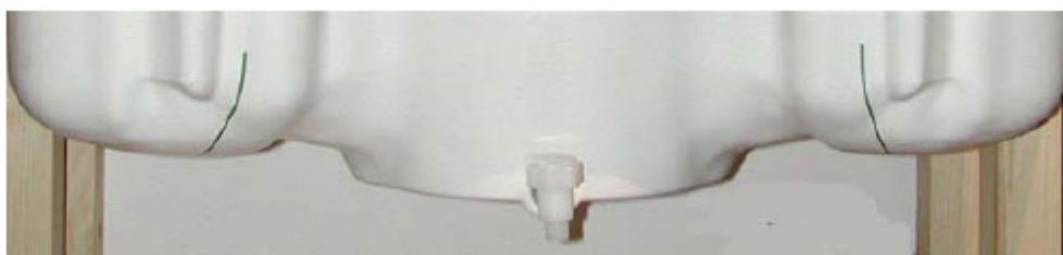
Figure 7.2 SAM Twin Phantom shell
