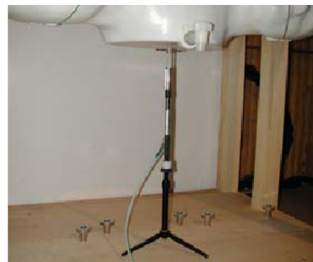
Figure 12.1 Dipole Validation Test Setup
