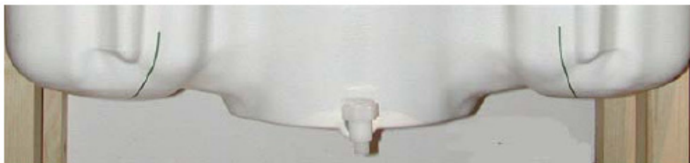
Figure 7.2 SAM Twin Phantom shell
