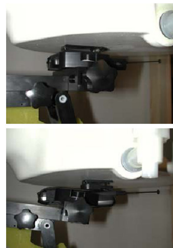
Figure 9.5 Body Belt Clip & Holster Configurations
