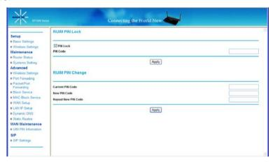
**RUIM PIN Lock:** Create a 4-digit PIN code, enter it into the "PIN Code" column box, and click "Apply".
