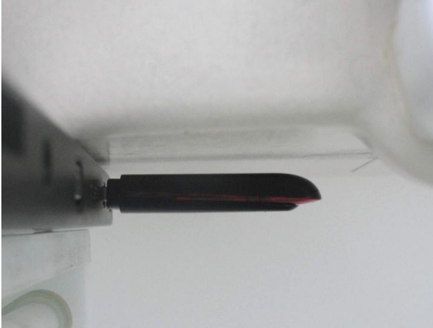
Direct Laptop Plug-in for USB Configuration 1 (Horizontal Up with Phantom 5 mm Gap)
