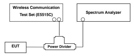
(Configuration of conducted Emission measurement)
