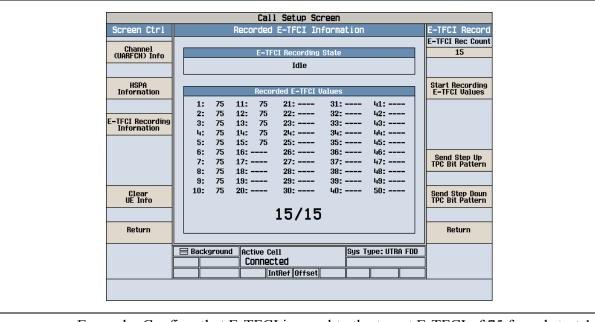
Example: Confirm that E-TFCI is equal to the target E-TFCI of 75 for sub-test 1
