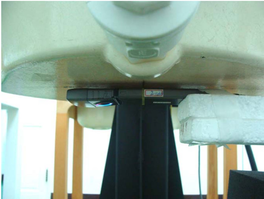
DUT Bottom with Phantom 0.5cm Gap (Antenna in Horizontal Position)
