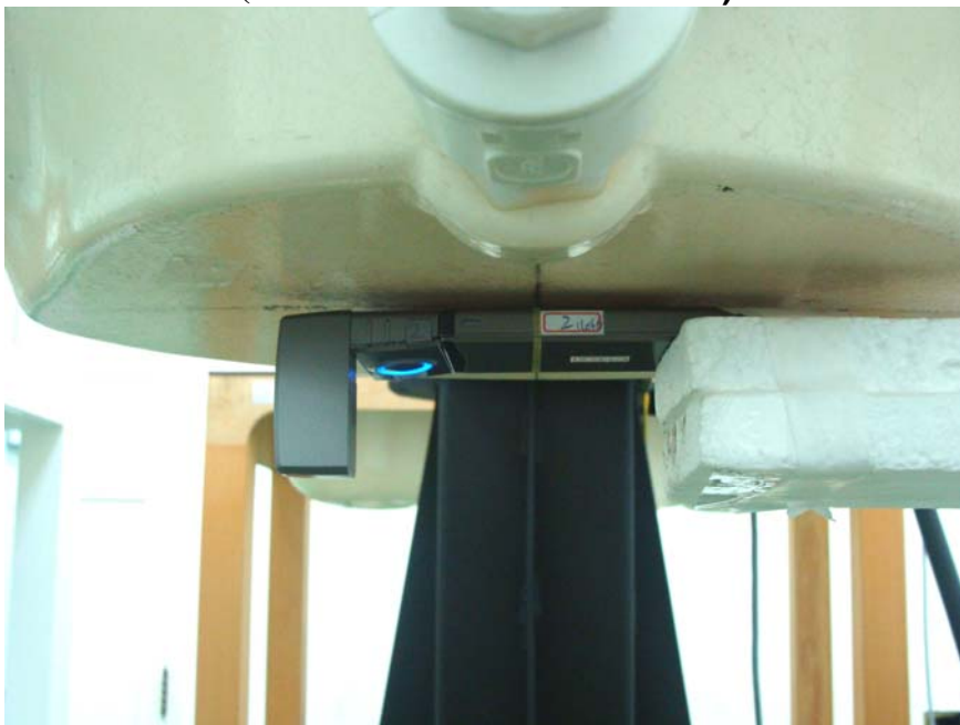
DUT Bottom with Phantom 0.5cm Gap (Antenna in Vertical Position)
