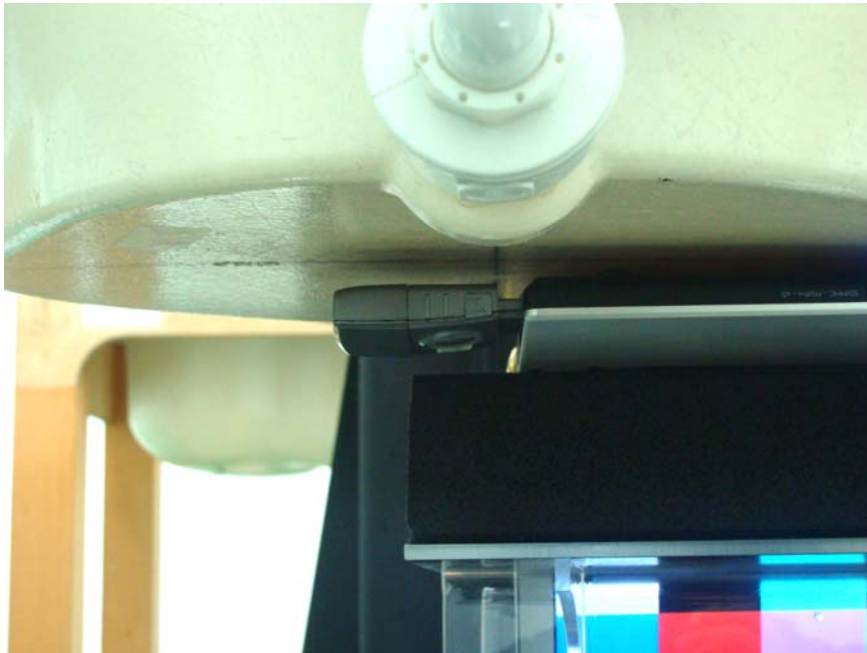
DUT Bottom with Phantom 1cm Gap (Antenna in Horizontal Position)
