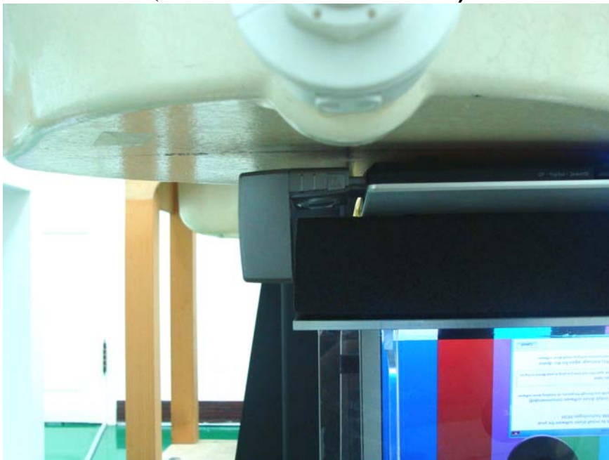
DUT Bottom with Phantom 1cm Gap (Antenna in Vertical Position)
