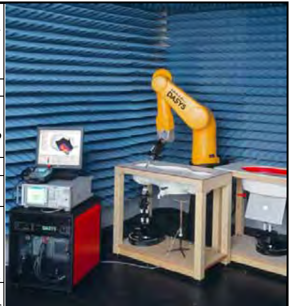
Fig. 5.2 Probe Setup on Robot
