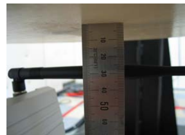
Fig. 21. Body SAR Test Setup with Holster
