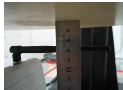
Fig. 21. Body SAR Test Setup with Holster
