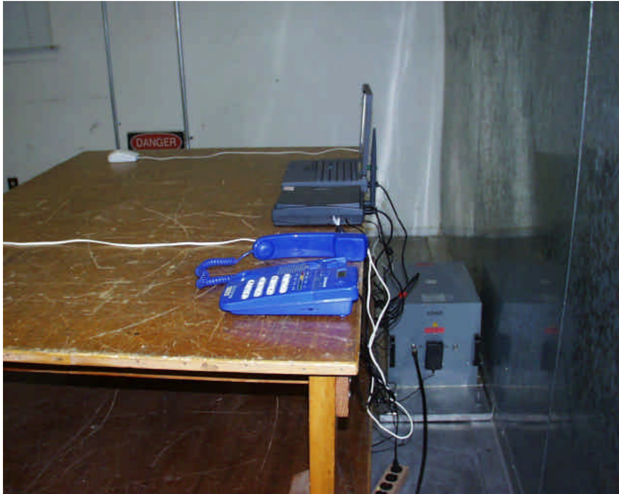
Conducted Emissions Setup, Rear View
