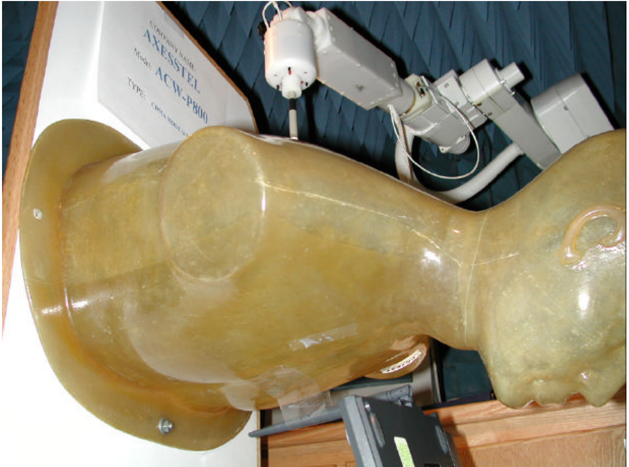
Fig. 8 Test Setup of EUT in operating position with the source of significant emissions (antenna) 2.54 cm below the phantom.
