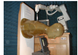
Fig. 1 SAR Test Setup
