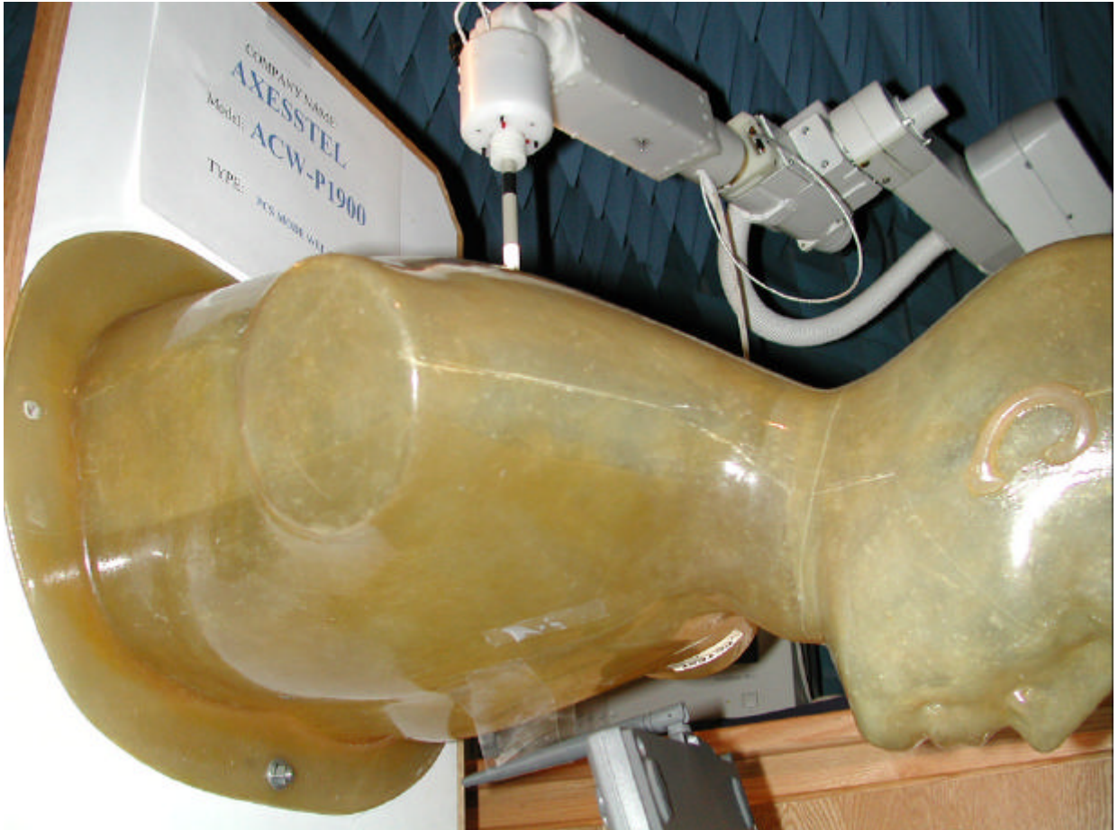
Figure 8. Test Setup of EUT in operating position with the source of significant emissions (antenna) 2.54 cm below the phantom.
