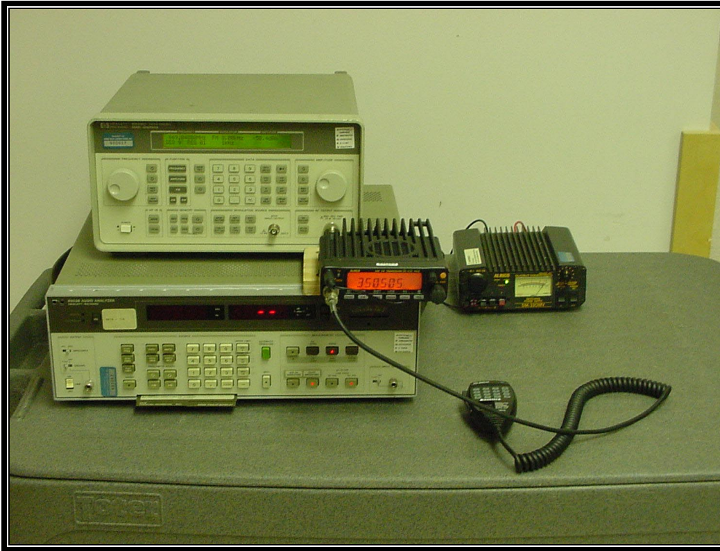
PHOTOGRAPH 6: 38 DB REJECTION SETUP
