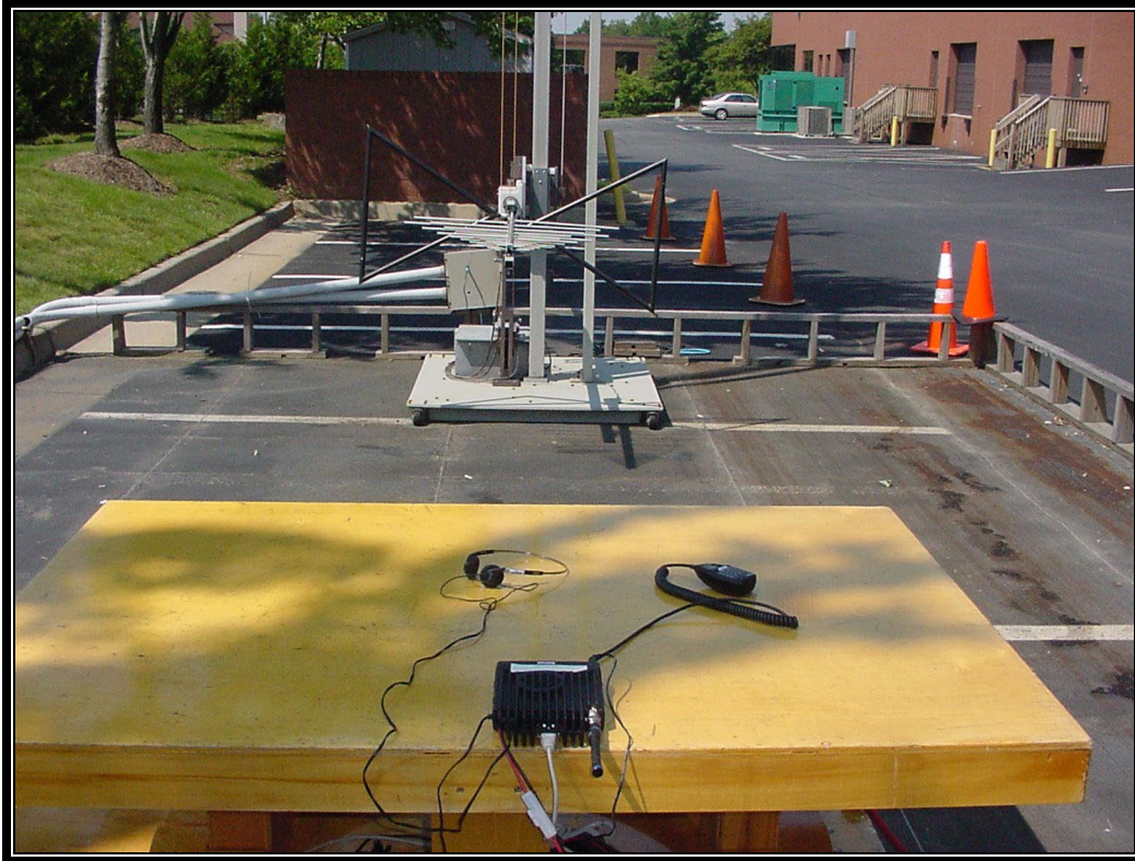
PHOTOGRAPH 5: RADIATED TEST CONFIGURATION (REAR VIEW)
