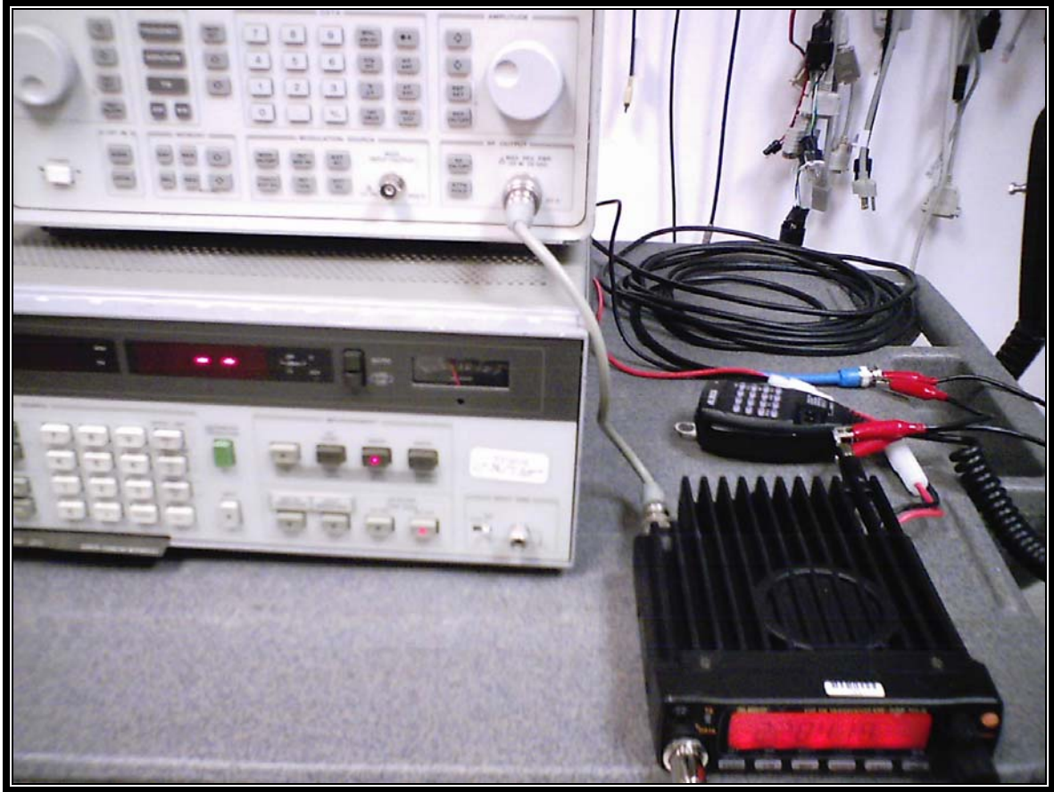
Photograph 6: 38 dB Rejection Test Setup
