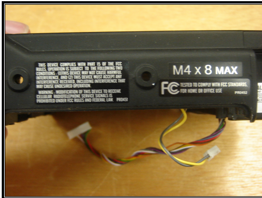
Photograph 2: Warning Label Location on End of EUT
