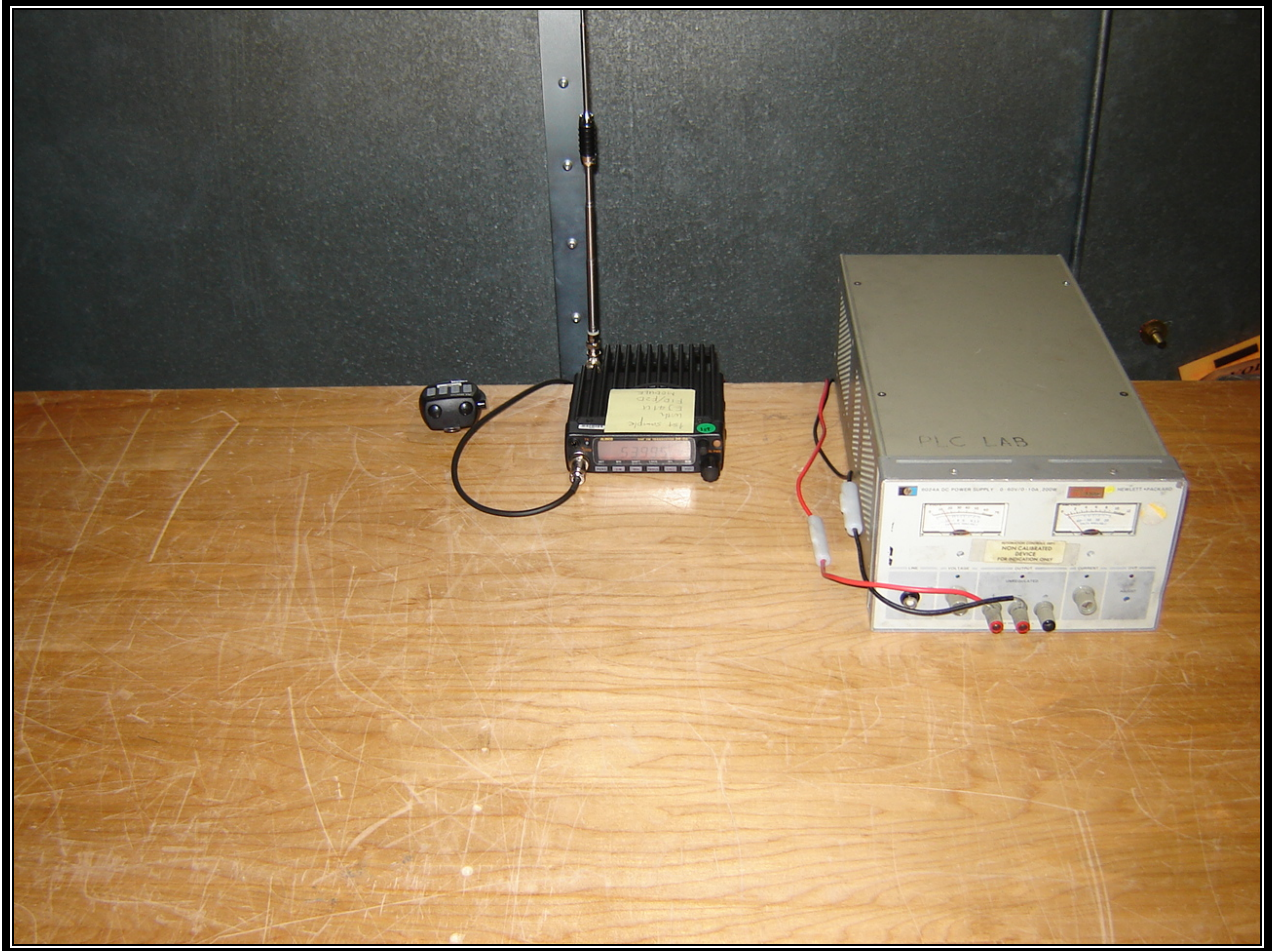
Photograph 6: Conducted AC Emissions Test Configuration (Front View)
