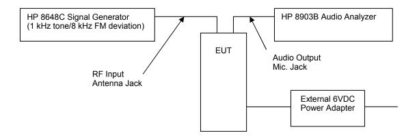
Frequencies used on the signal generator were 824.04, 836.50, and 848.97 MHz for the mobile band, and 869.04, 881.50, and 893.97 MHz for the base band.
