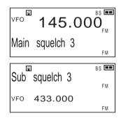
Rotating the dial clockwise sets the squelch level higher; rotating the dial counterclockwise sets the squelch level lower.
