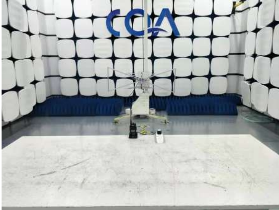
Radiated emission Test Setup (30MHz~1GHz)
