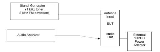
Frequencies used on the signal generator were 824.04, 836.50, and 848.97 MHz for the mobile band, and
