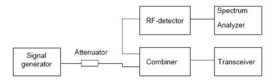
For equipment with intergal antenna the connector to the equipment is made either to a temporary 50 ohm Connector, the spectrum analyzer is operated in zero span mode and the resolution bandwith shall be approximately 3 times the channel bandwith.
