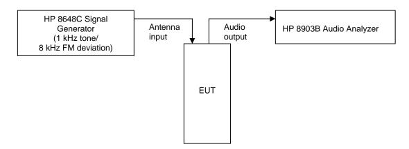
Frequencies used on the signal generator were 824.04, 836.50, and 848.97 MHz for the mobile band, and 869.04, 881.50, and 893.97 MHz for the base band.
