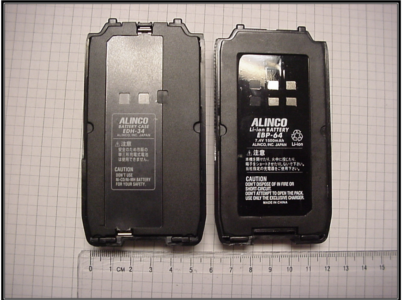
Photograph 16: EDH-34, EBP-64 Battery Labels
