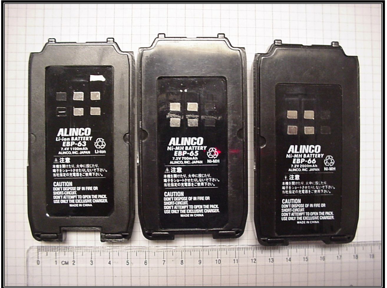
Photograph 15: EBP-63, EBP-65, EBP-66 Battery Labels
