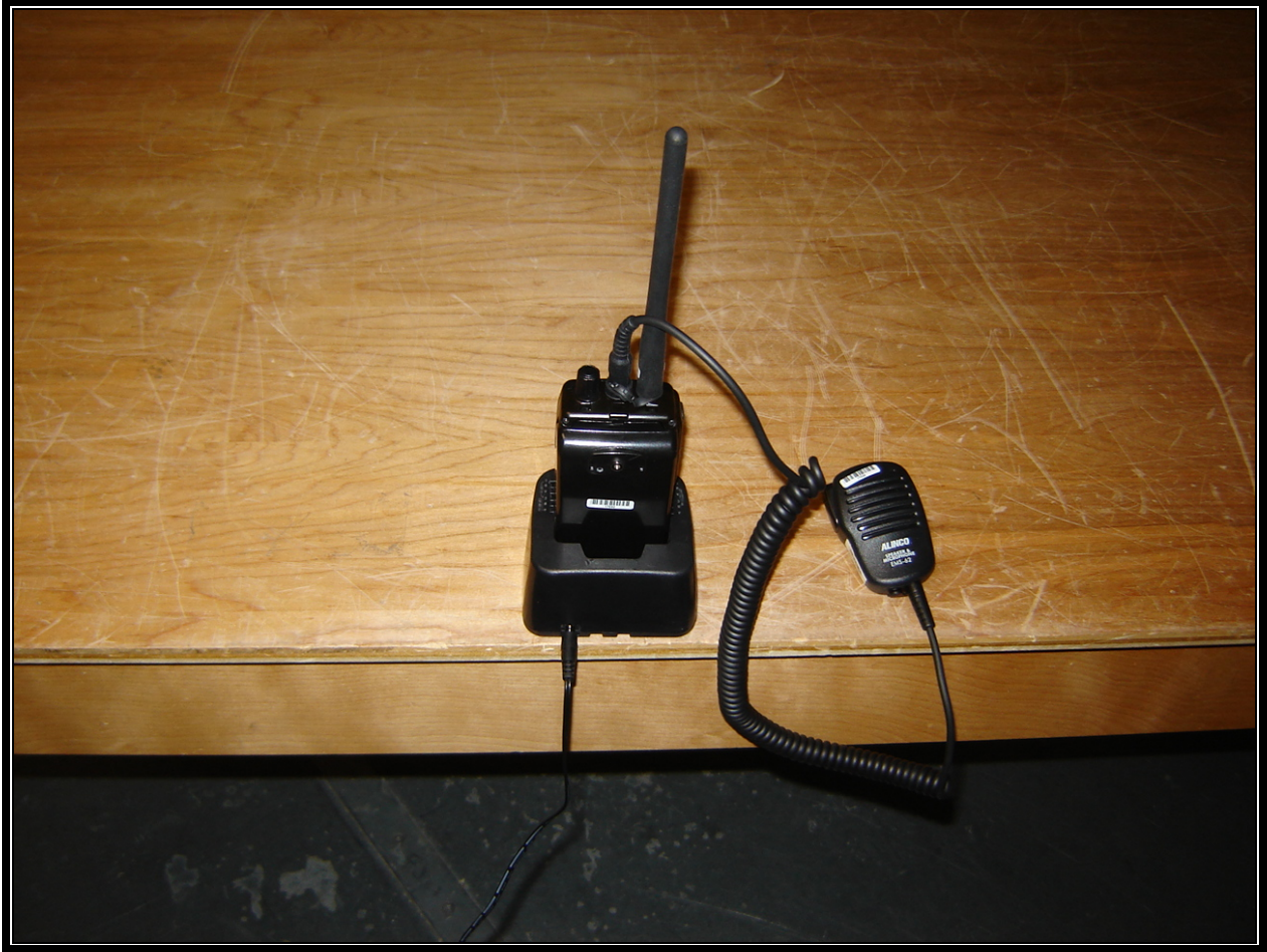
Photograph 7: Conducted AC Emissions Test Configuration (Rear View)
