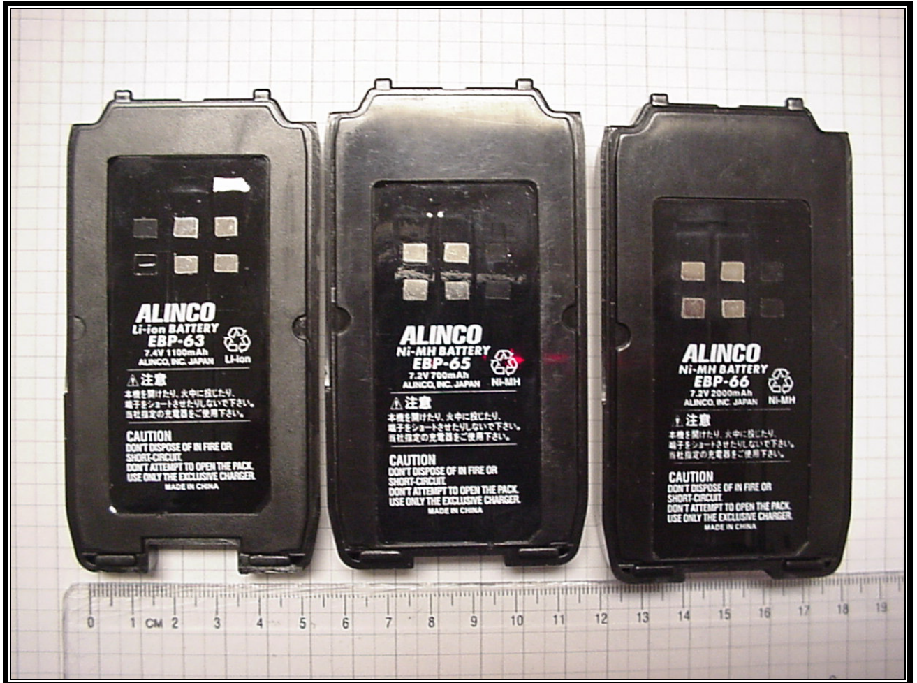
Photograph 13: EBP-63, EBP-65, EBP-66 Battery Labels
