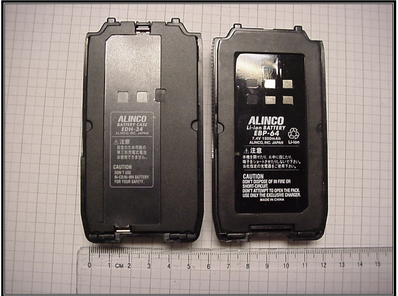
Photograph 14: EDH-34, EBP-64 Battery Labels
