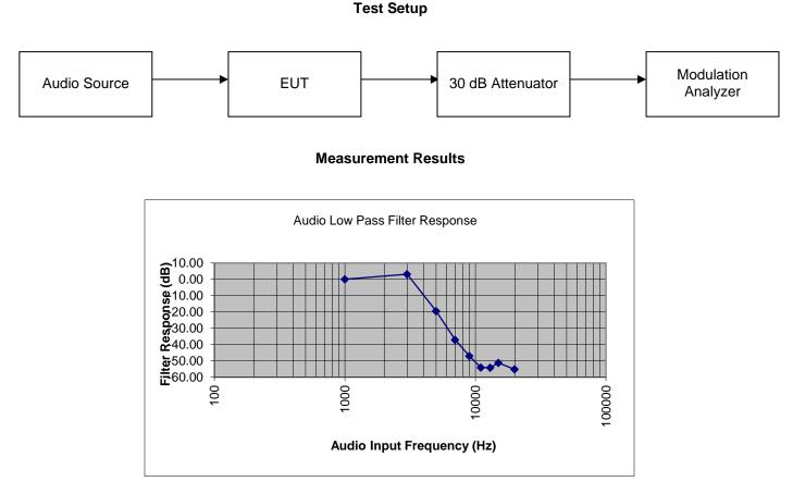
This unit is a digital radio and the roll-off for the filter is very linear in the operational band and sharp out of band.
