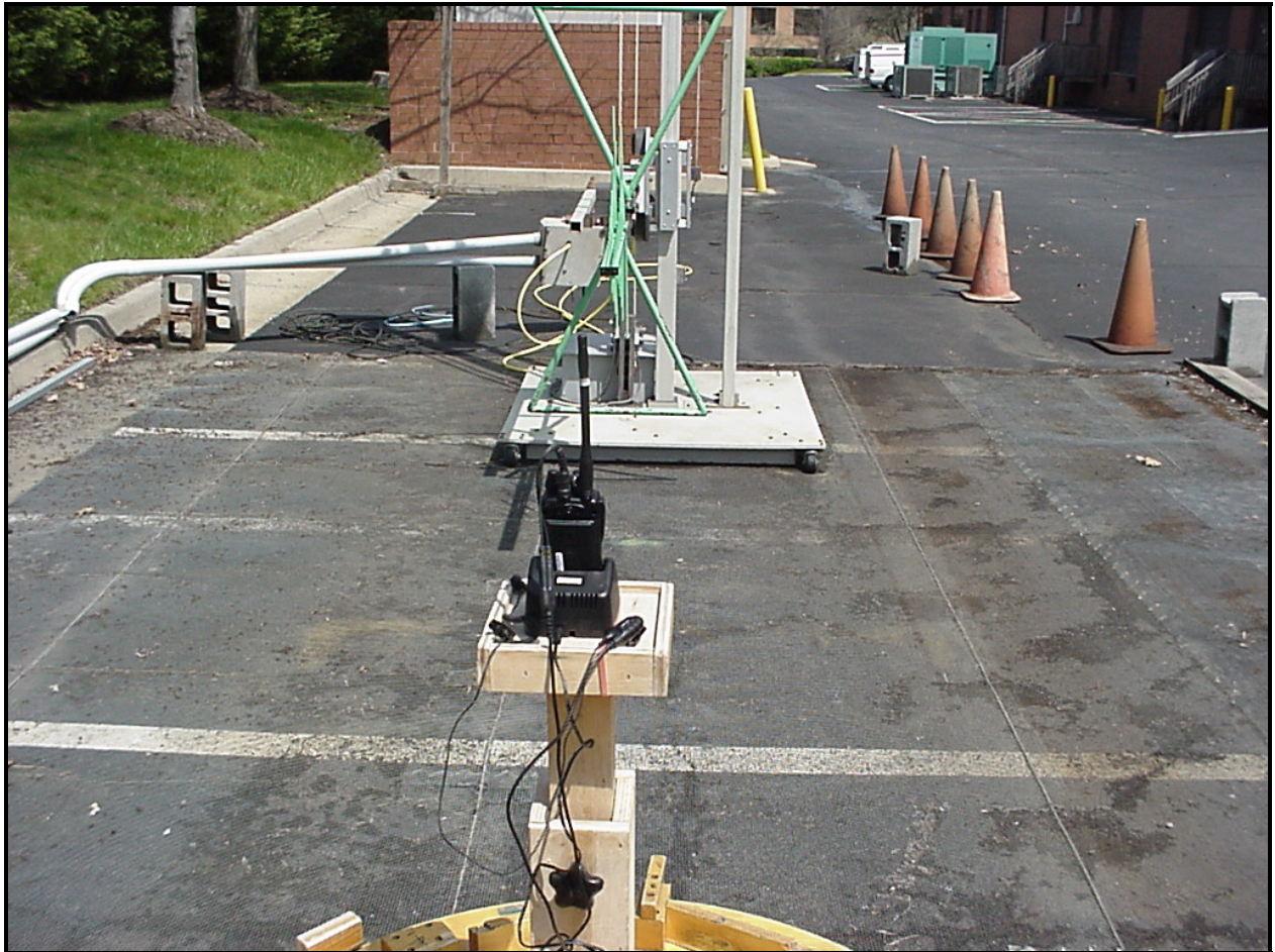
Photograph 3: Radiated Emissions Test Configuration (Rear View)
