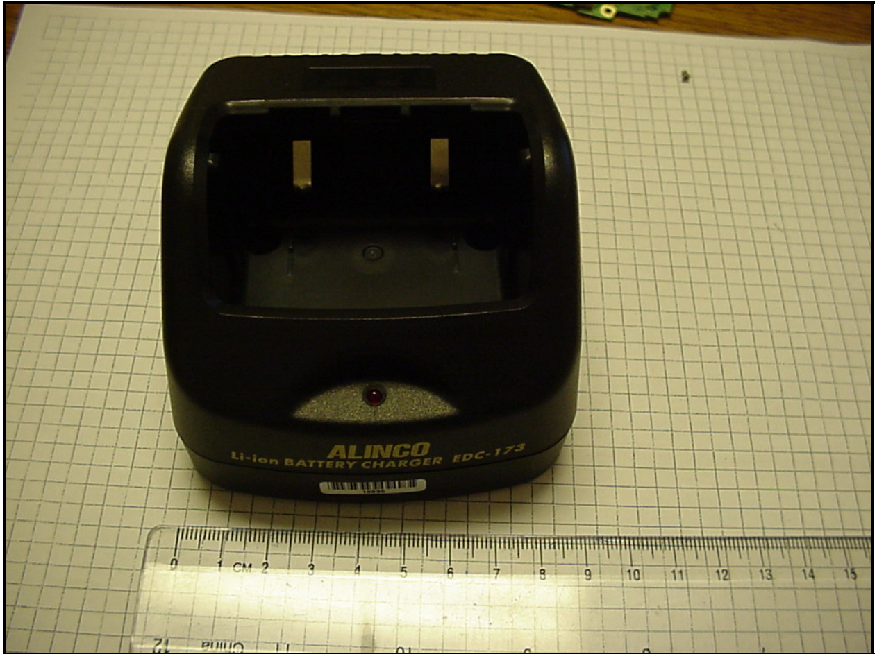
Photograph 16: EDC-173 Battery Charger
