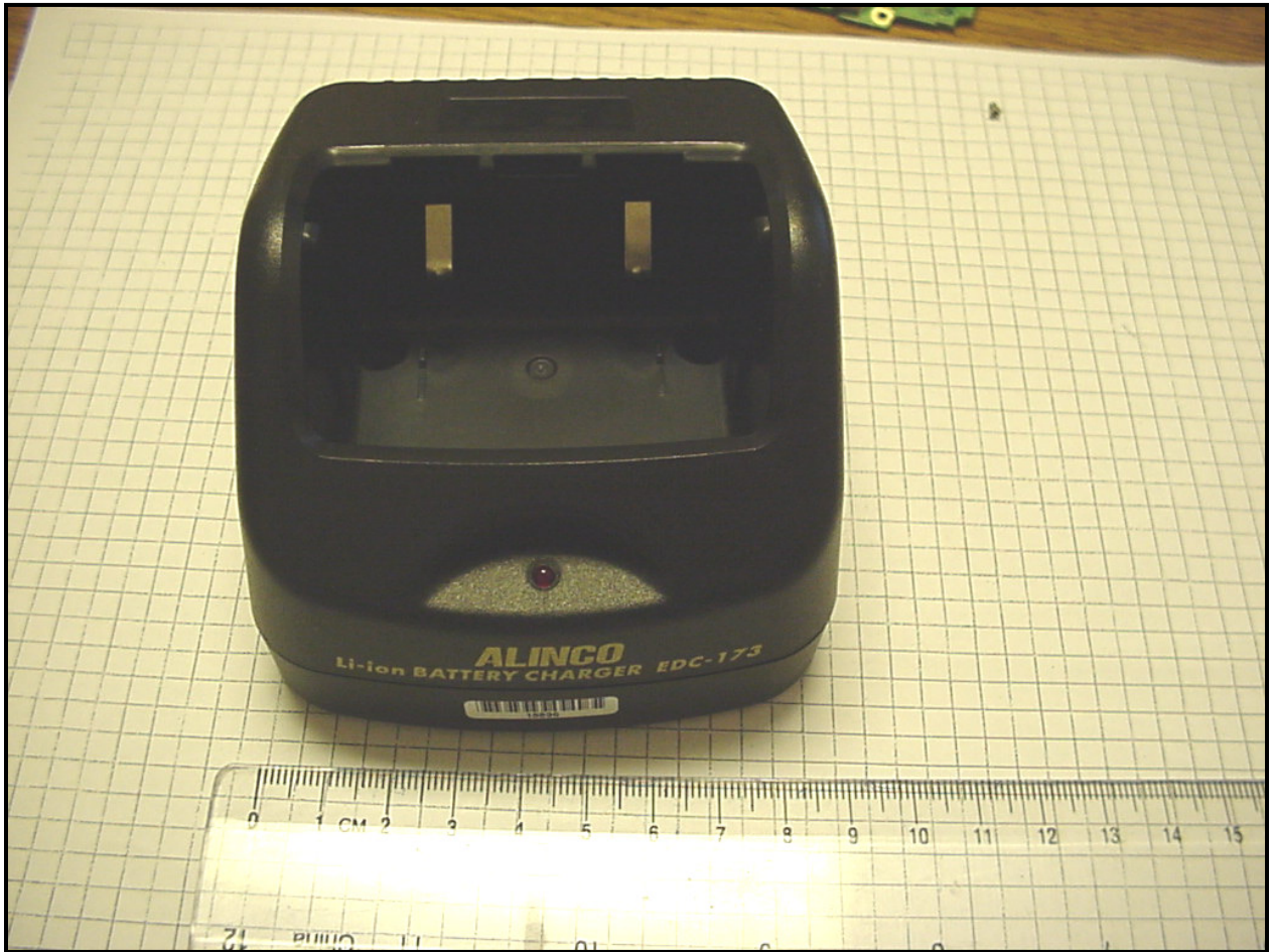
Photograph 16: EDC-173 Battery Charger
