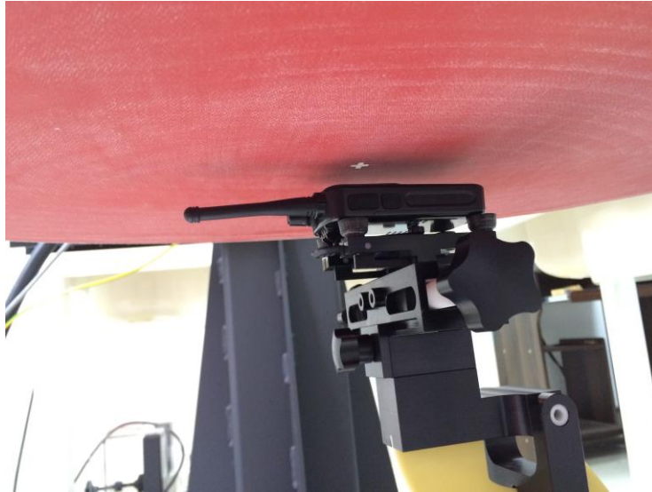
Face-held, the front of the EUT towards phantom (The distance was 25mm)
