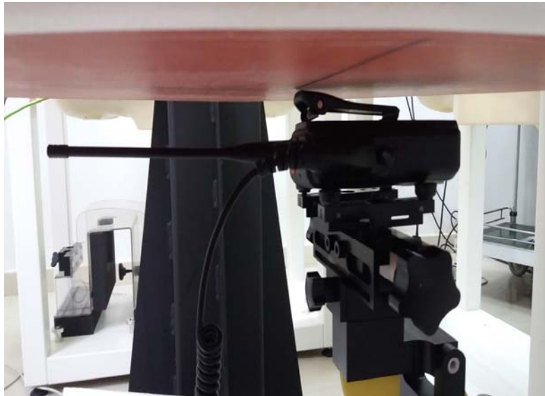
Body-worn, the front of the EUT towards ground with A1, B1 and D1 (The distance was 0mm)
