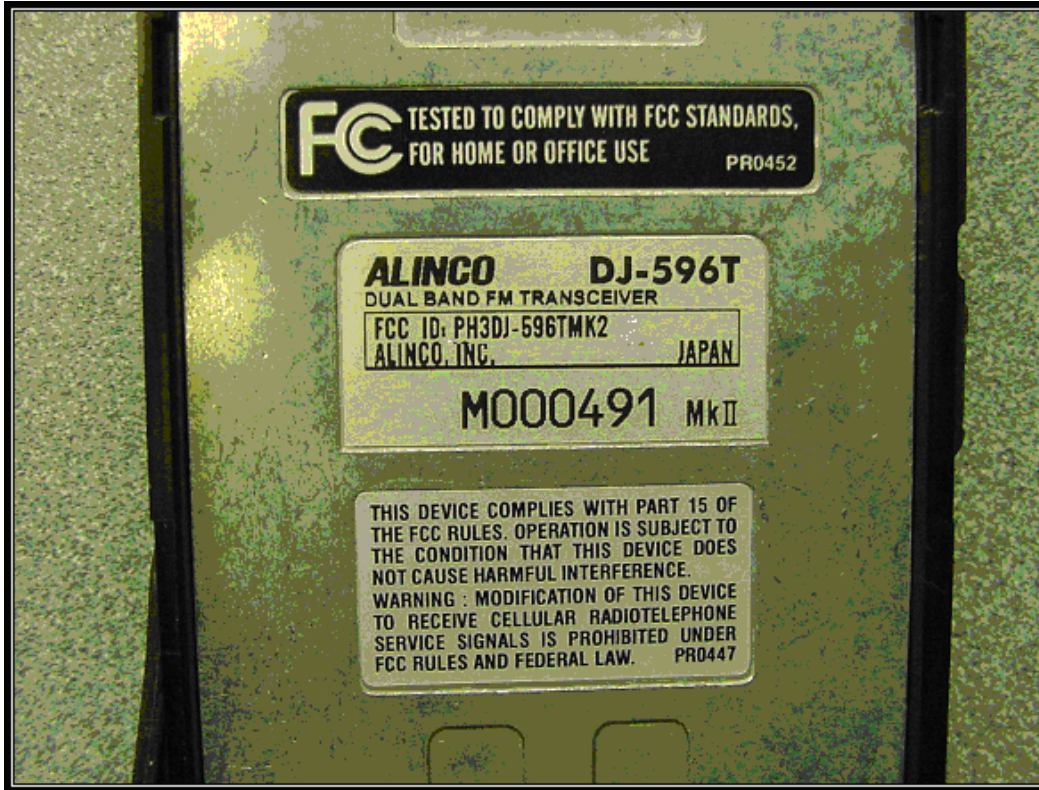
PHOTOGRAPH 1: FCC ID LABEL AND WARNING LABEL SHOWN ON THE BACK OF EUT (without battery pack)
