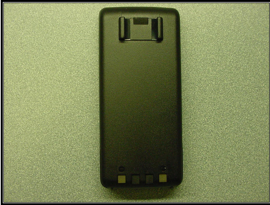
PHOTOGRAPH 12: BOTTOM OF BATTERY PACK
