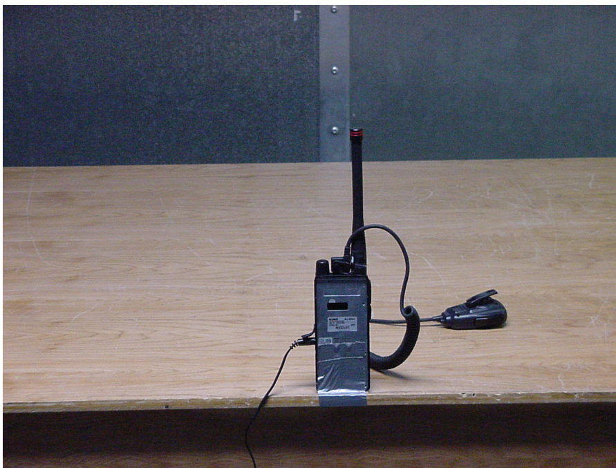
PHOTOGRAPH 3: CONDUCTED TEST CONFIGURATION (REAR VIEW)
