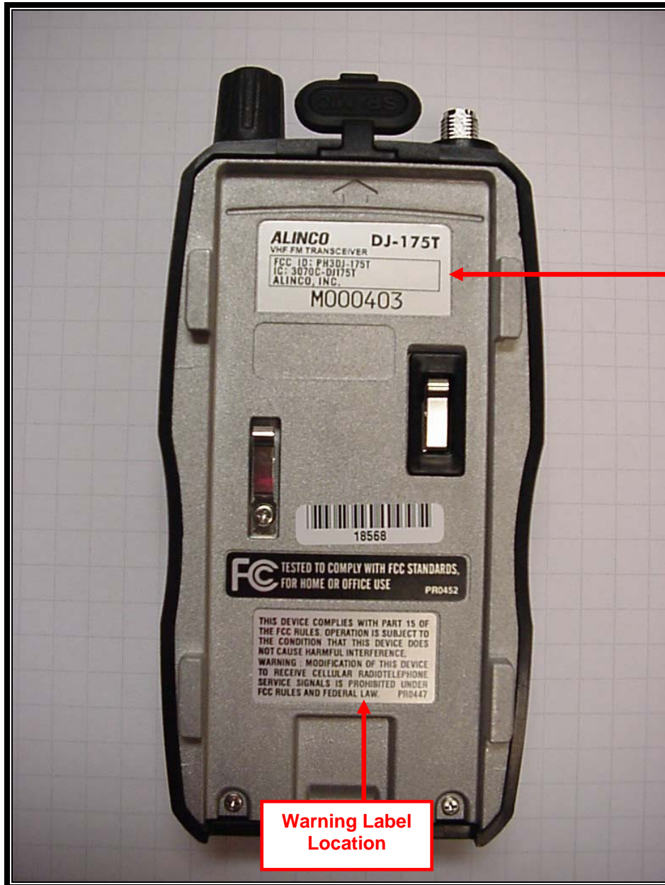
Photograph 1: FCC/IC ID and Warning Label Locations
