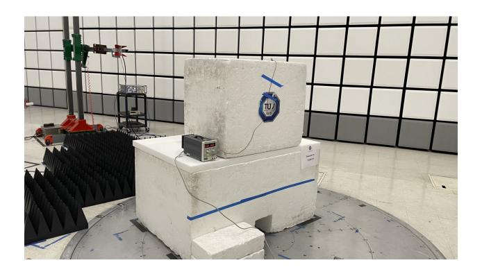
Radiated Emissions Test Setup (1GHz to 18GHz)
