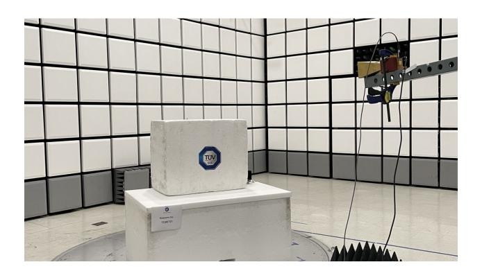
Radiated Emissions Test Setup (18GHz to 26GHz)
