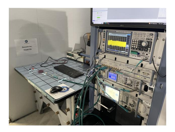
**Antenna Conducted Port Test Setup**
