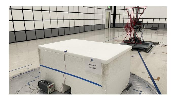
Radiated Emissions Test Setup (30MHz to 1GHz)
