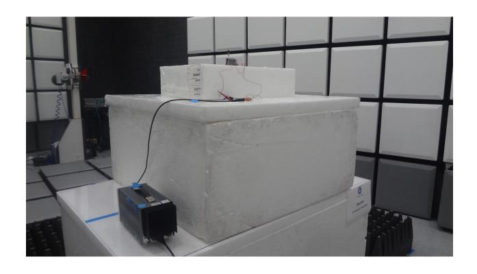
Radiated Emissions Test Setup (1GHz to 18GHz)
