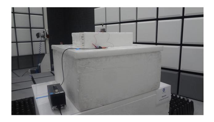
Radiated Emissions Test Setup (above 18GHz)
