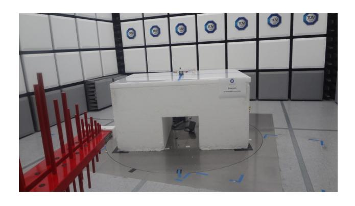
Radiated Emissions Test Setup (30MHz to 1GHz)
