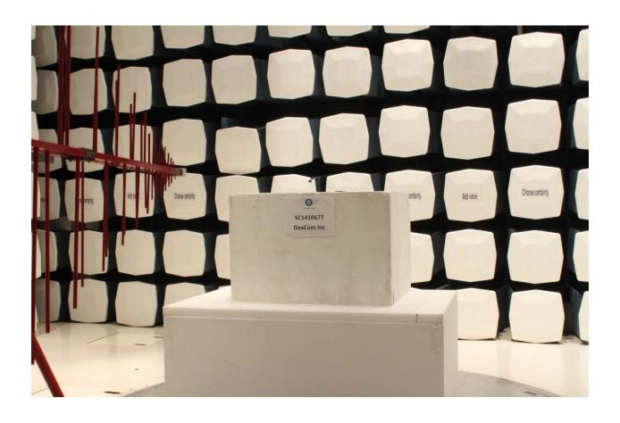
Radiated Emissions Test Setup (below 1GHz)
