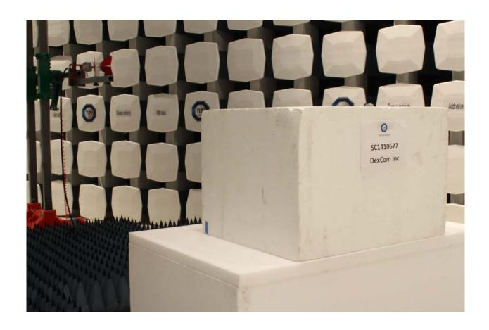
Radiated Emissions Test Setup (above 1GHz)
