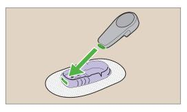
Slide transmitter tab into the slot at the narrow end of the holder.
