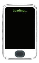
Press and hold **power button** for 2 seconds to turn receiver on. Wait for loading screen to appear.
