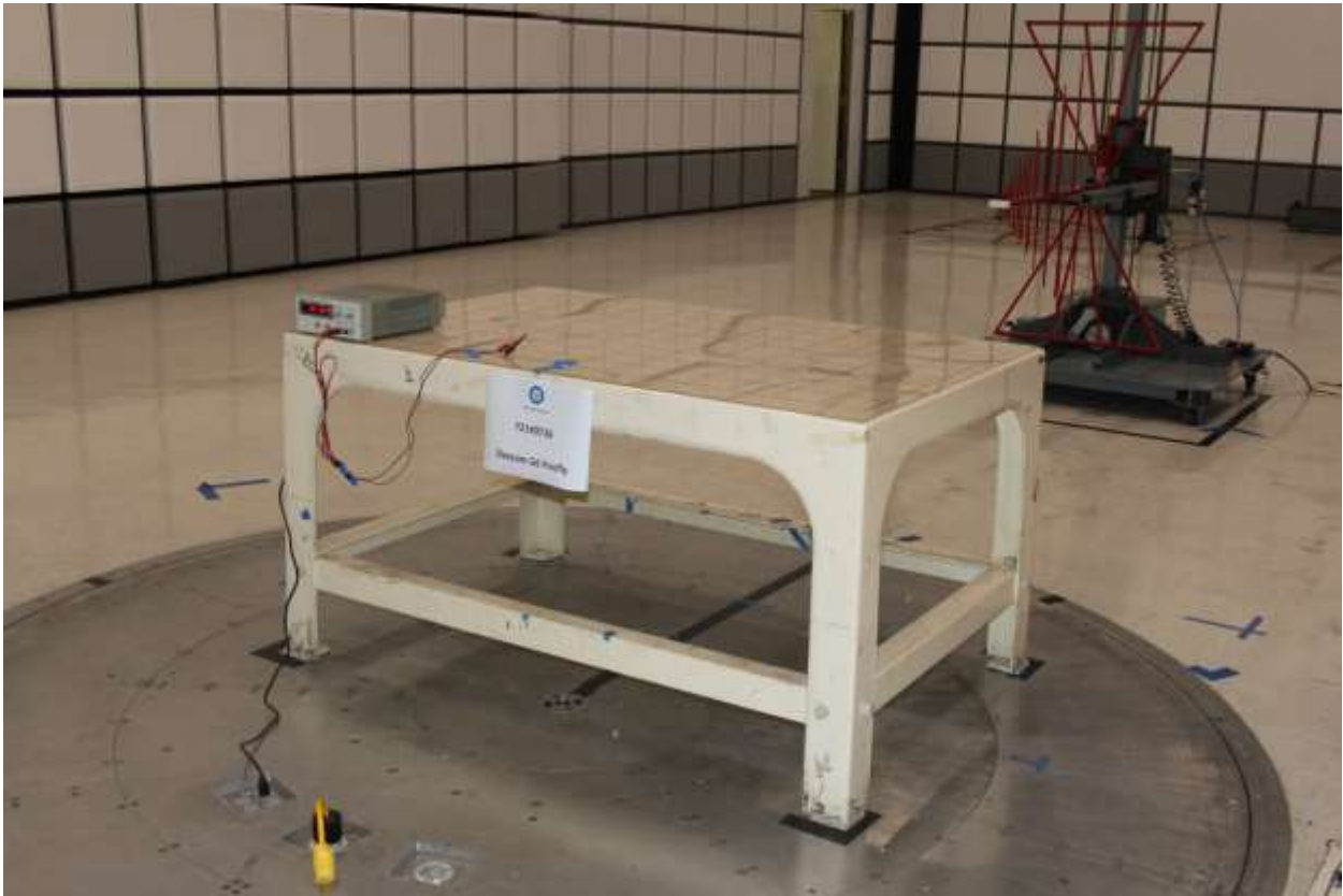
Radiated Emissions Test Setup (below 30MHz)
