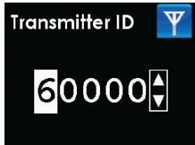
Transmitter ID setting screen, first digit highlighted
