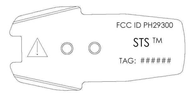
Label is physically engraved into the bottom of each STS Transmitter.
