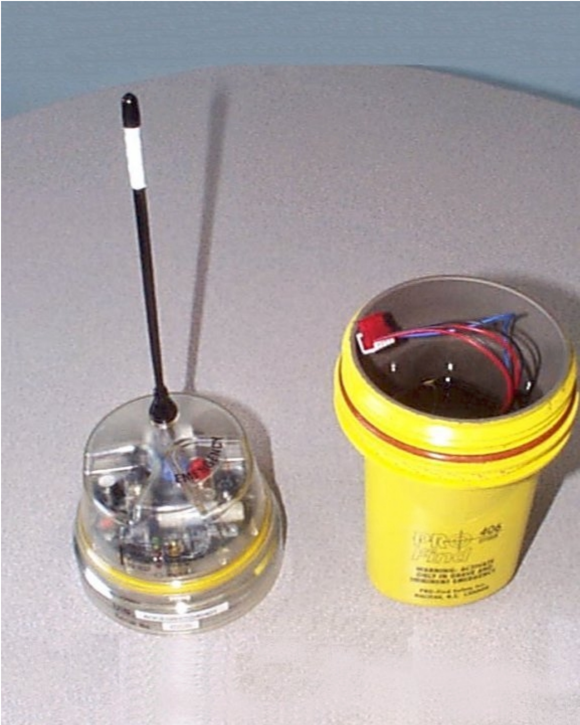
Photograph 4. EPIRB and Battery
