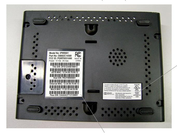
Position base serial-number label (middle section of **D888-IPW9001-Product-Label-RevB)** as squarely as possible in position shown.
