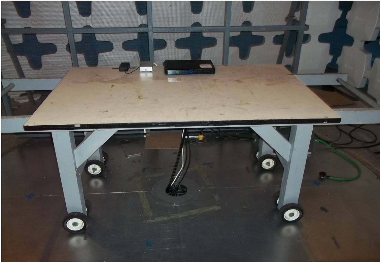
Test Configuration Photograph #1 (Conducted Emissions - Power Port)
