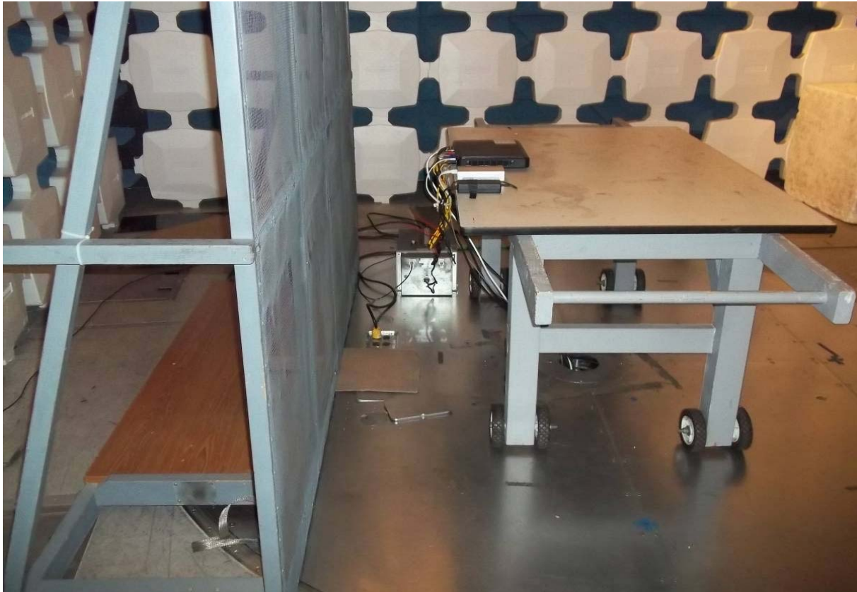
Test Configuration Photograph #2 (Conducted Emissions - Power Port)
