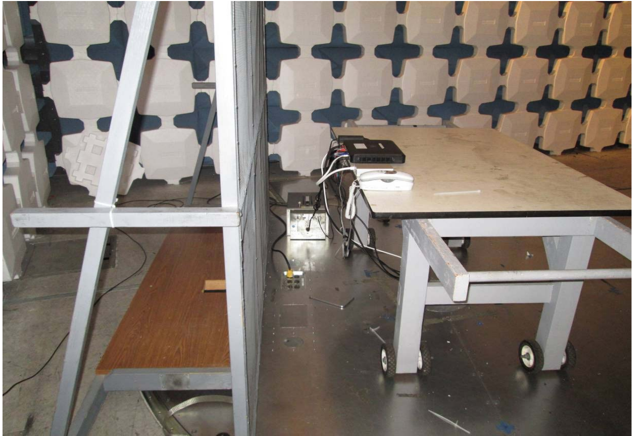
Test Configuration Photograph #2 (Conducted Emissions - Power Port)
