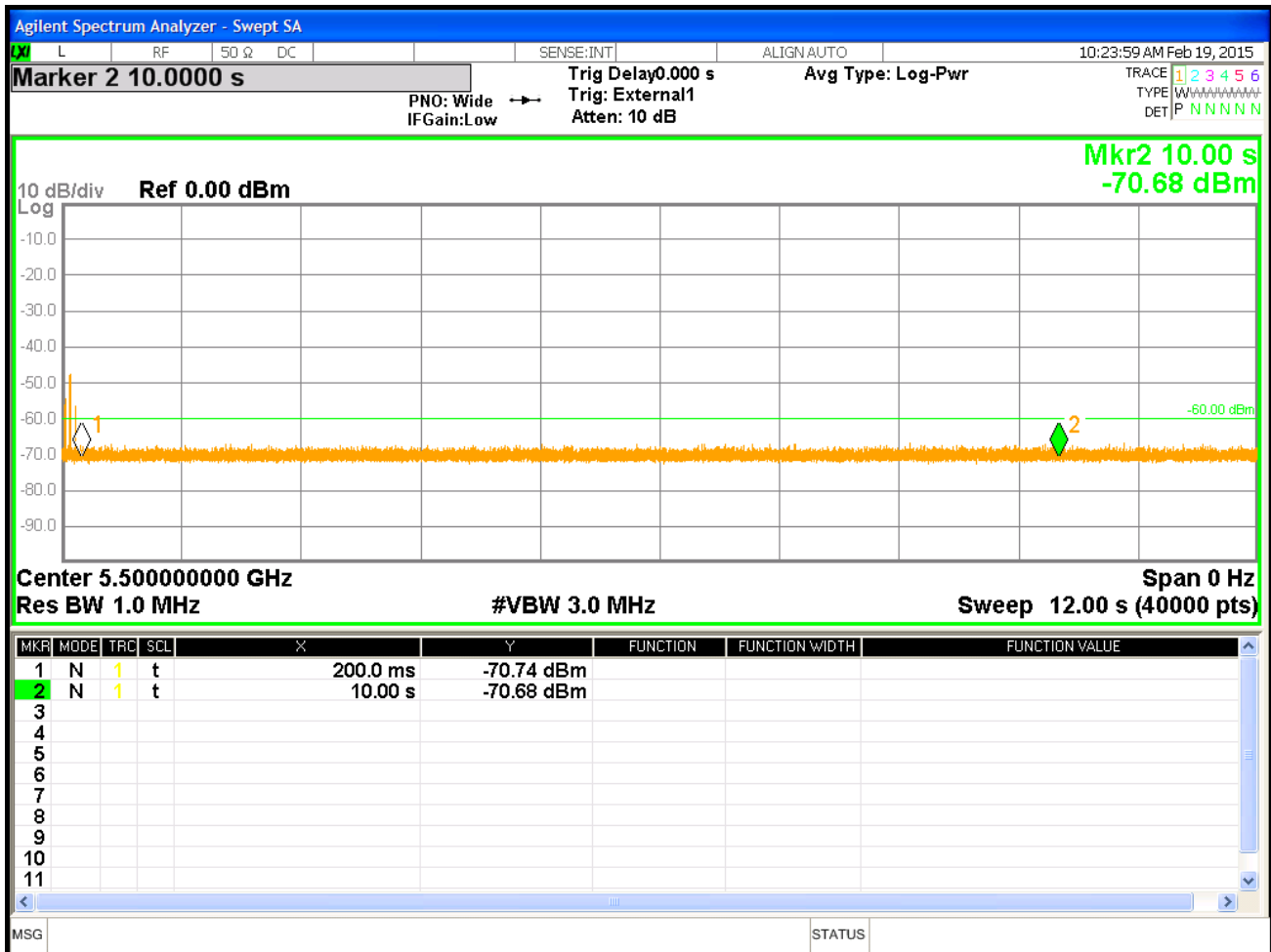
Figure 2: Channel move time, signal plotted 10 secs after radar signal is applied at 5500 MHz for 20MHz BW
