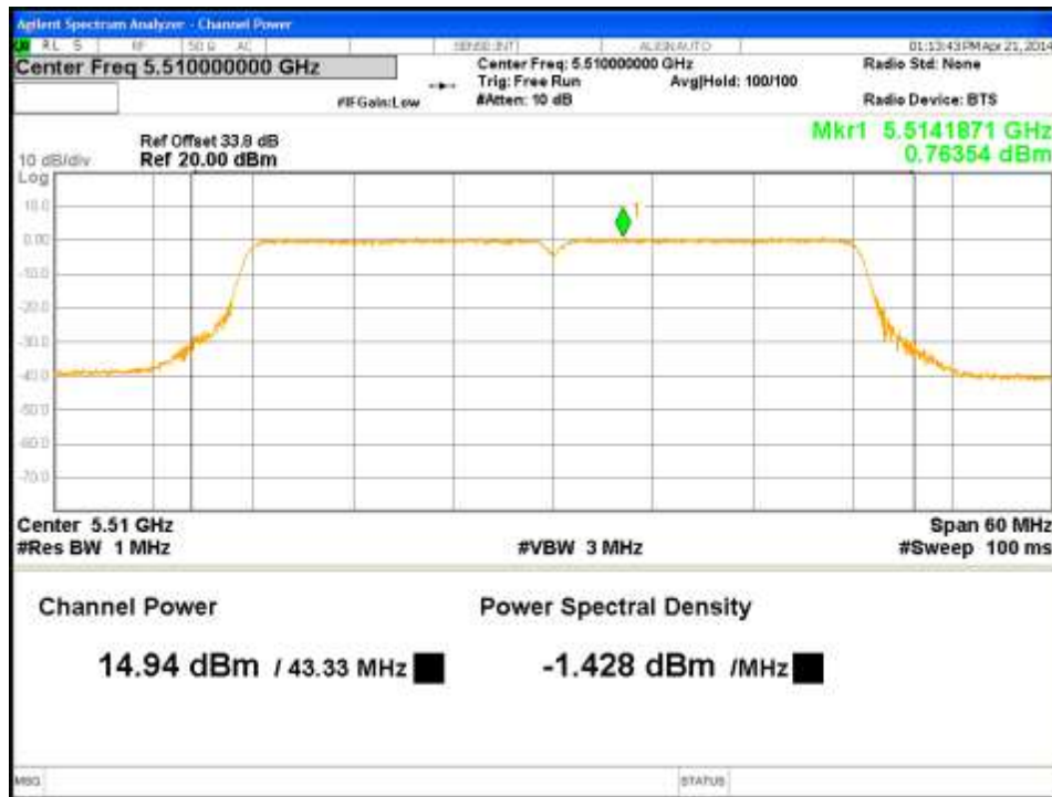
Figure 25: Maximum Conducted Output Power-5510MHz-HT40-MCS0-Ch0
