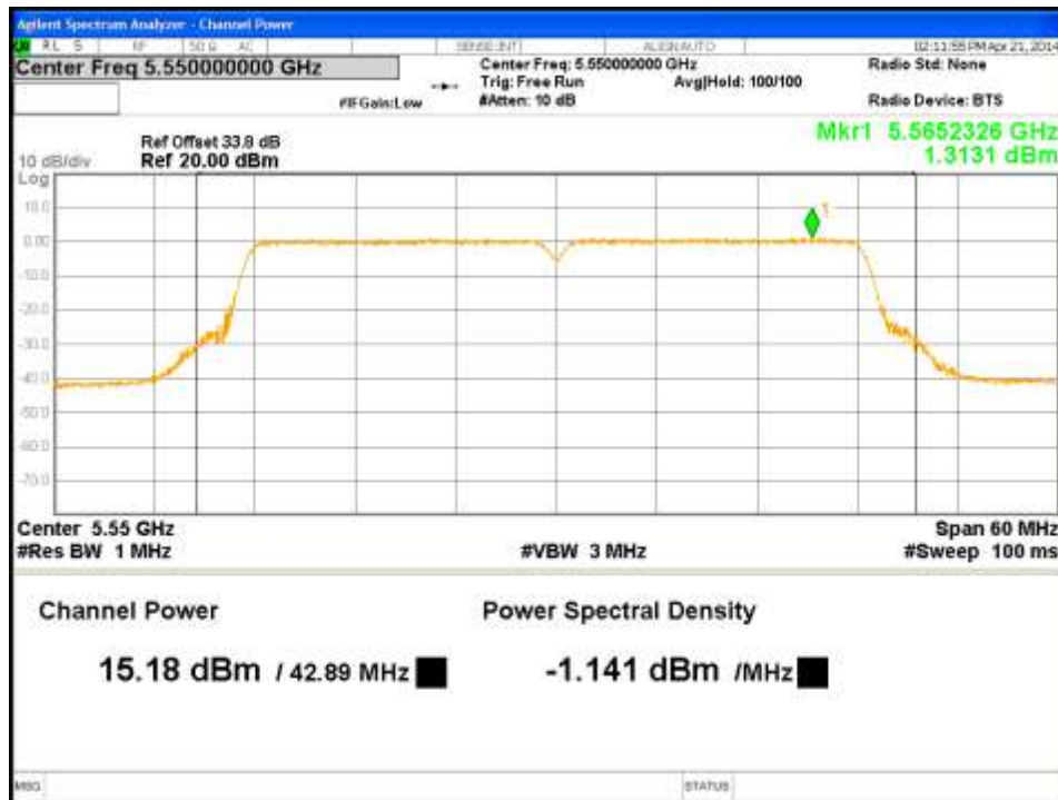
Figure 55: Maximum Conducted Output Power-5550MHz-VHT40-MCS0-Ch2
