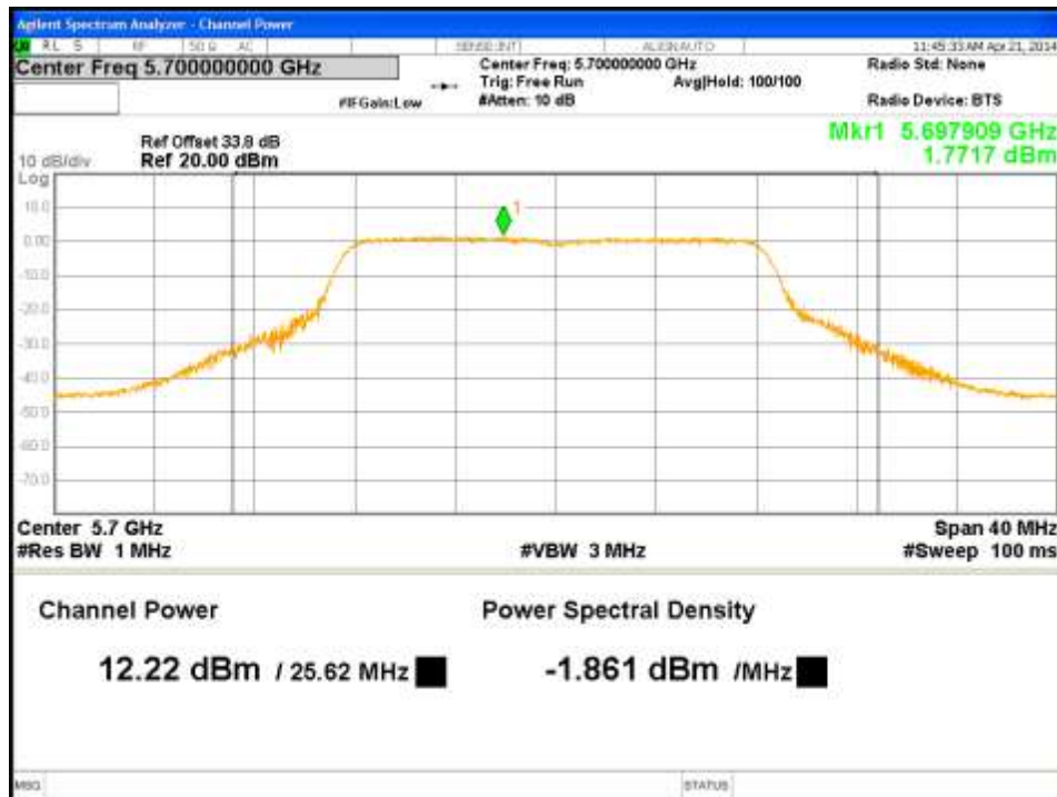
Figure 10: Maximum Conducted Output Power-5700MHz-11a-6Mbps-Ch1
