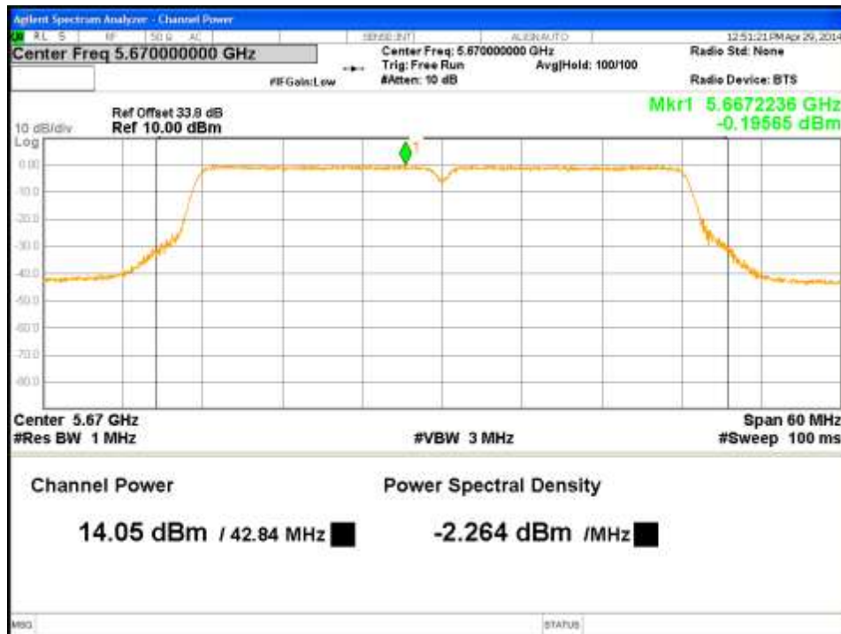
Figure 58: Maximum Conducted Output Power-5670MHz-VHT40-MCS0-Ch1
