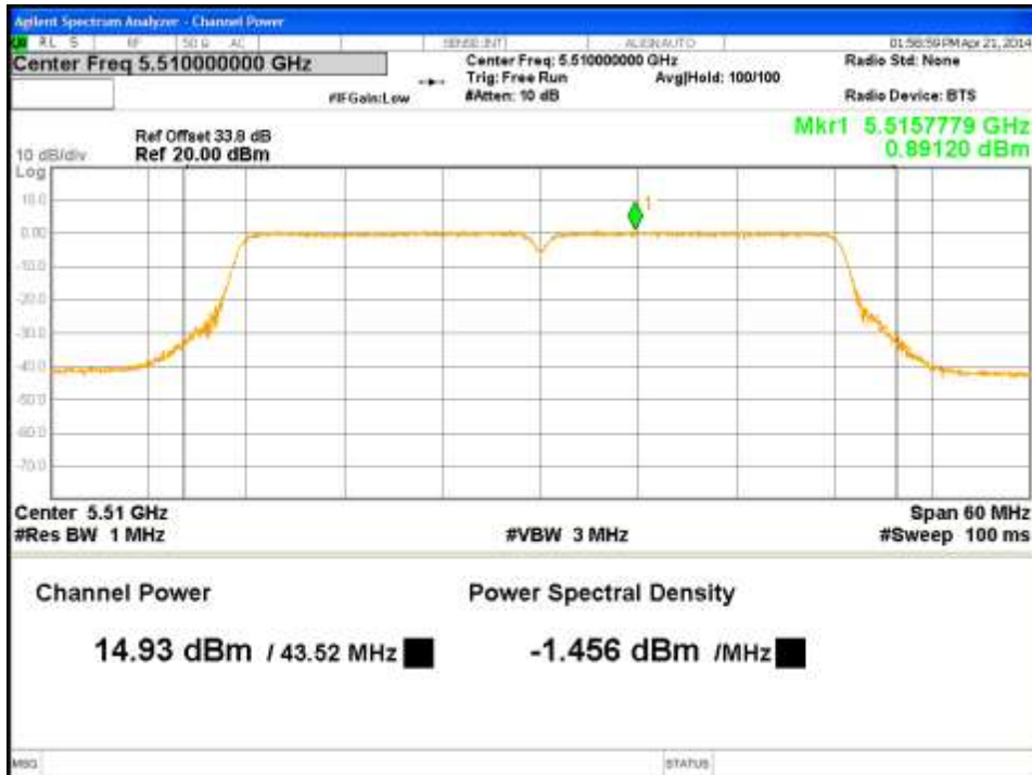
Figure 52: Maximum Conducted Output Power-5510MHz-VHT40-MCS0-Ch3
