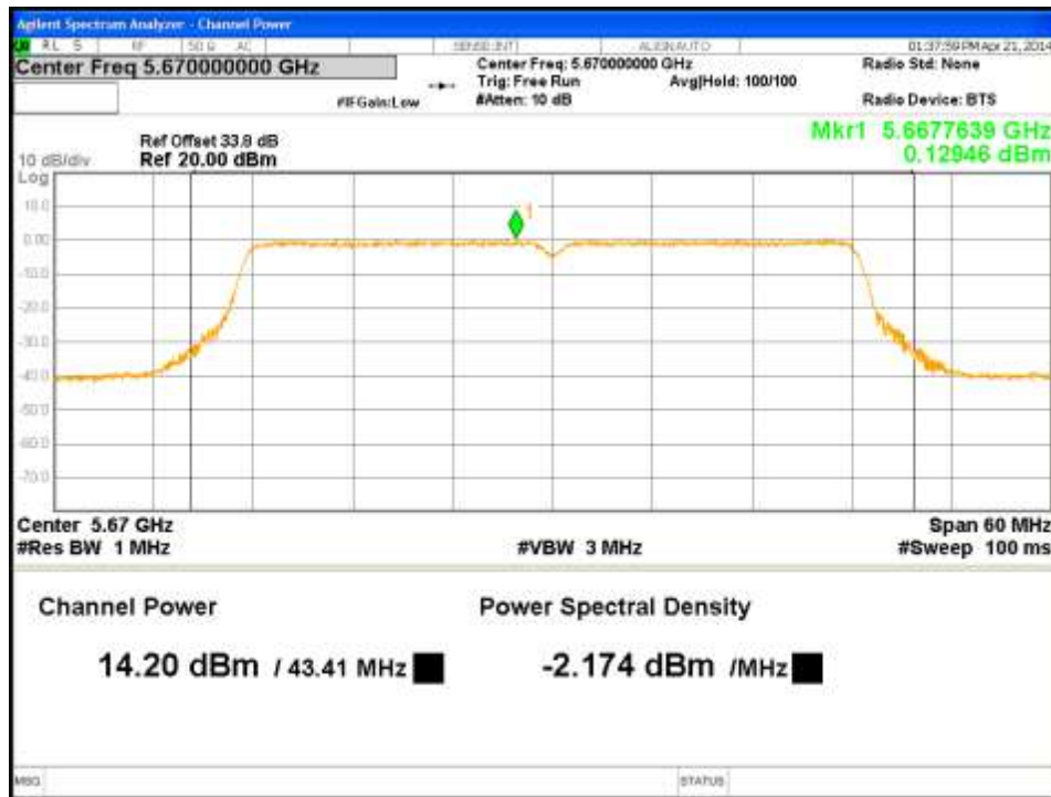
Figure 33: Maximum Conducted Output Power-5670MHz-HT40-MCS0-Ch0
