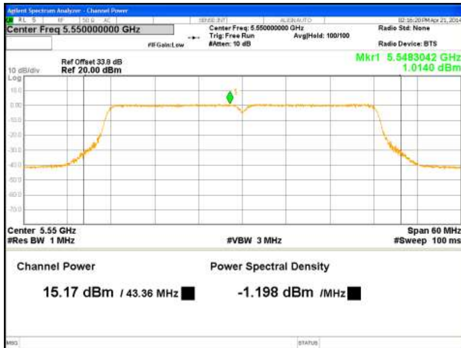
Figure 56: Maximum Conducted Output Power-5550MHz-VHT40-MCS0-Ch3
