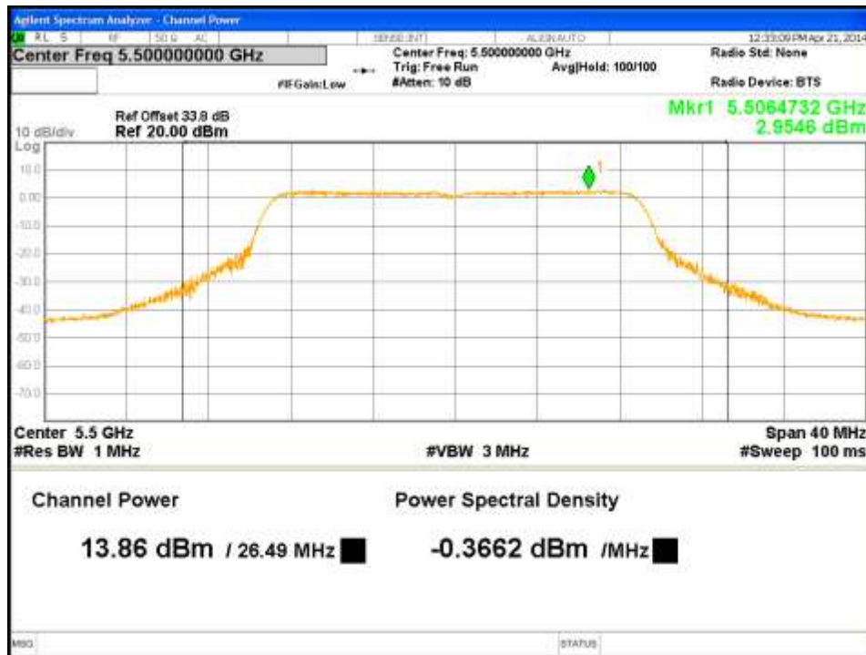
Figure 39: Maximum Conducted Output Power-5500MHz-VHT20-MCS0-Ch2
