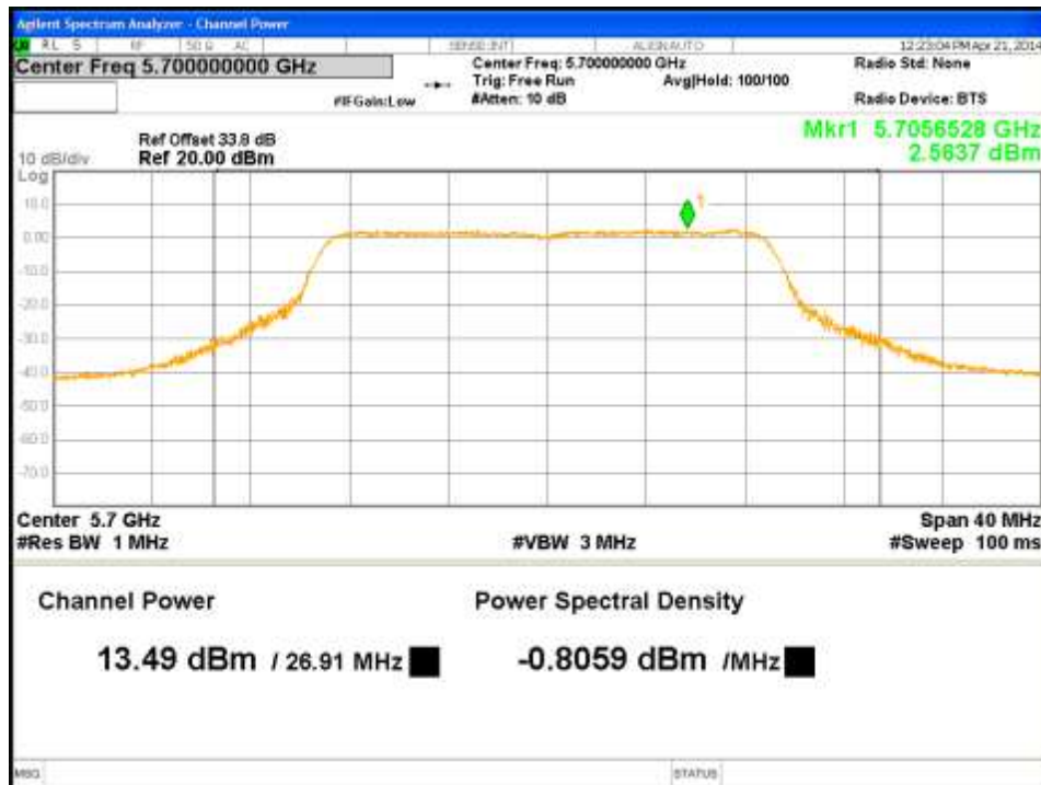
Figure 24: Maximum Conducted Output Power-5700MHz-HT20-MCS0-Ch3
