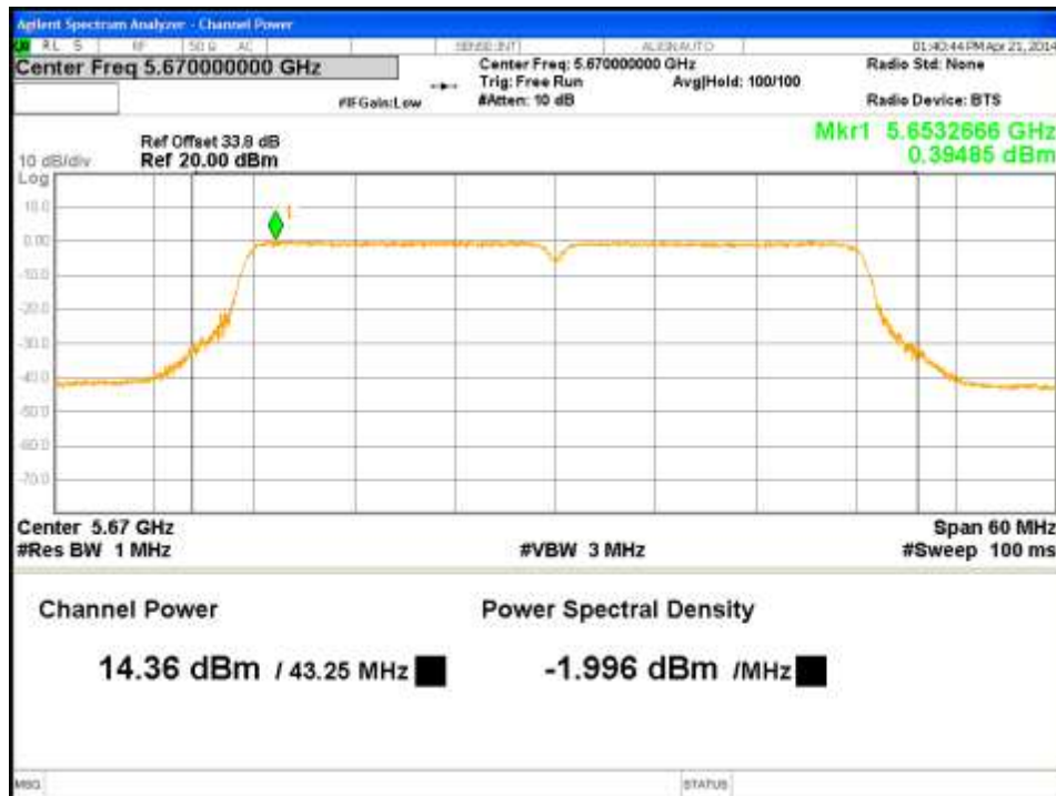
Figure 34: Maximum Conducted Output Power-5670MHz-HT40-MCS0-Ch1
