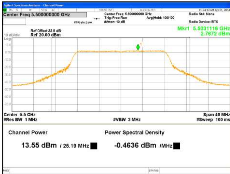
Figure 3: Maximum Conducted Output Power-5500MHz-11a-6Mbps-Ch2
