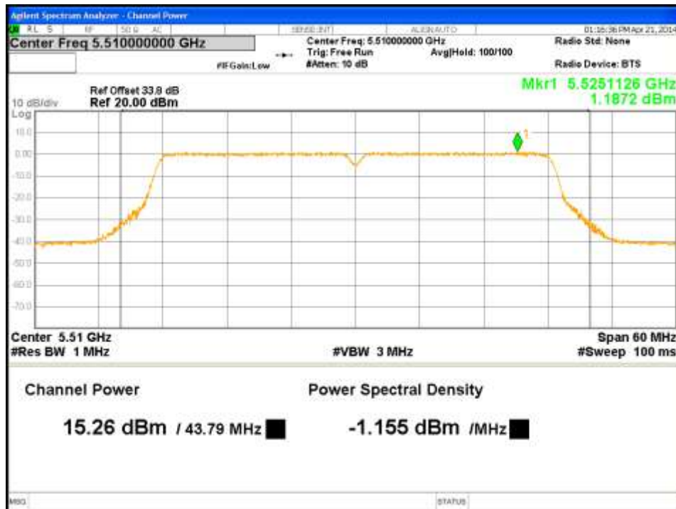
Figure 26: Maximum Conducted Output Power-5510MHz-HT40-MCS0-Ch1
