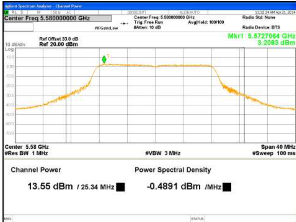
Figure 6: Maximum Conducted Output Power-5580MHz-11a-6Mbps-Ch1
