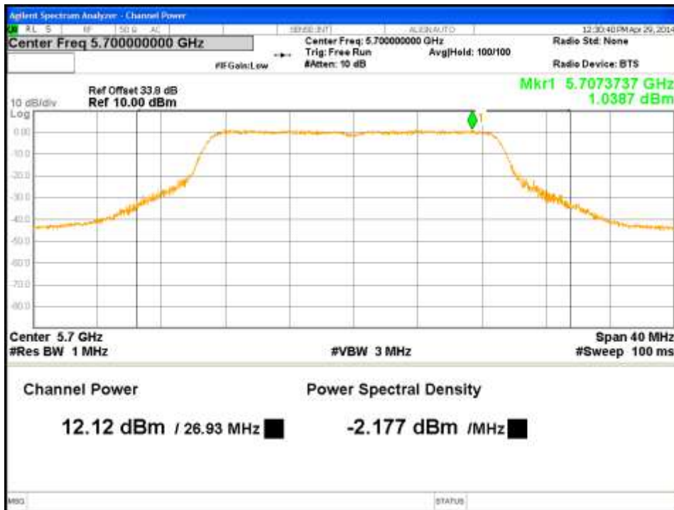
Figure 47: Maximum Conducted Output Power-5700MHz-VHT20-MCS0-Ch2
