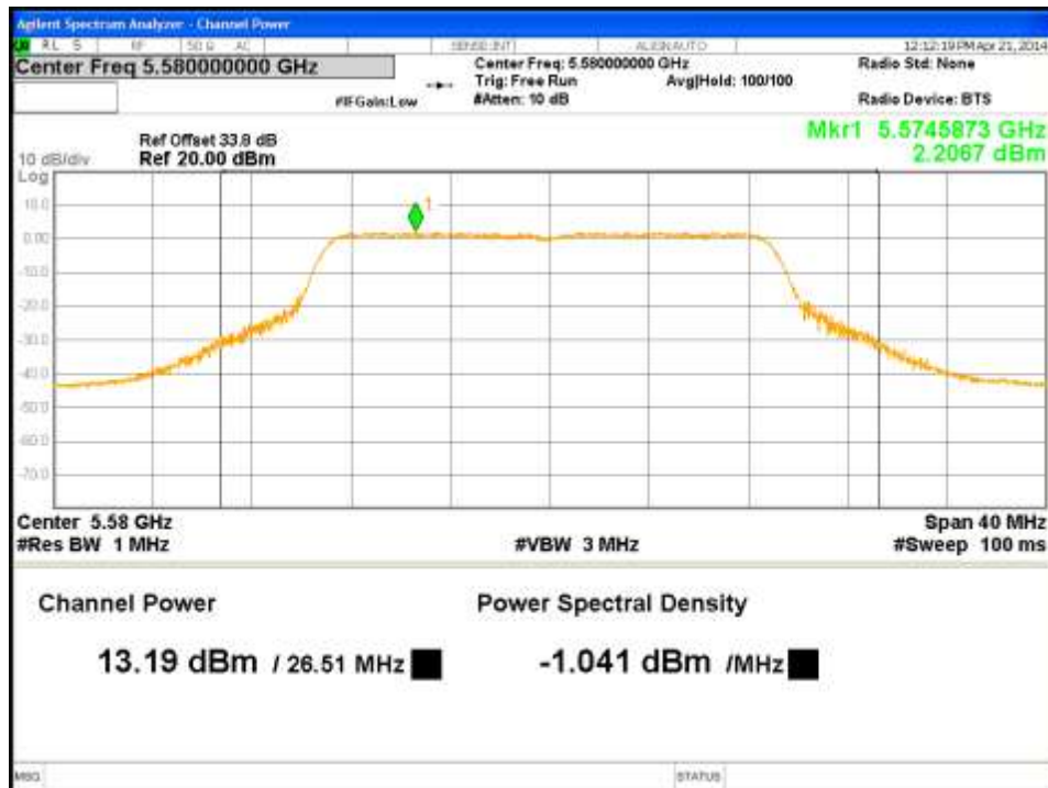
Figure 20: Maximum Conducted Output Power-5580MHz-HT20-MCS0-Ch3
