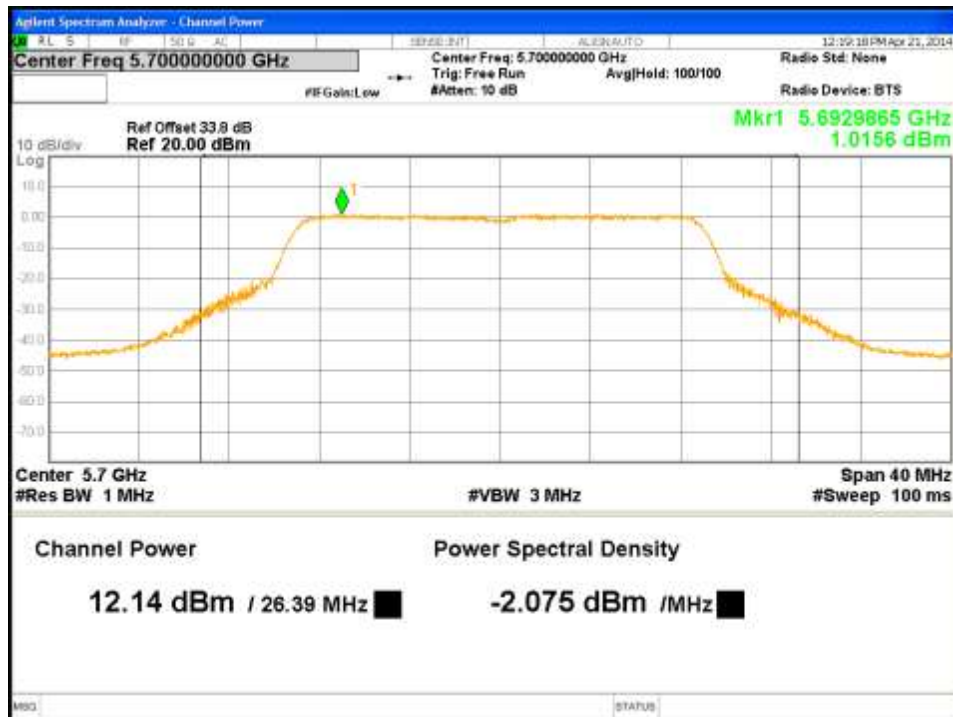
Figure 22: Maximum Conducted Output Power-5700MHz-HT20-MCS0-Ch1
