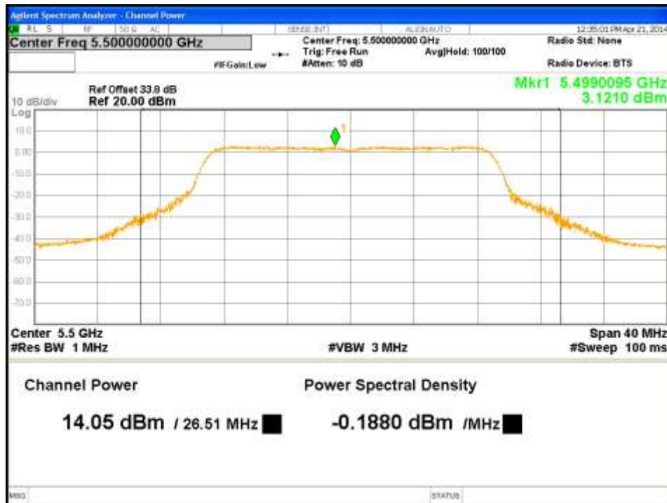
Figure 40: Maximum Conducted Output Power-5500MHz-VHT20-MCS0-Ch3
