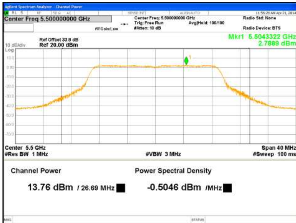
Figure 14: Maximum Conducted Output Power-5500MHz-HT20-MCS0-Ch1
