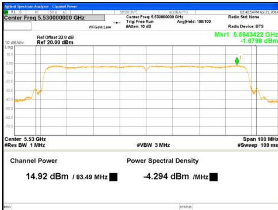
Figure 64: Maximum Conducted Output Power-5530MHz-VHT80-MCS0-Ch3
