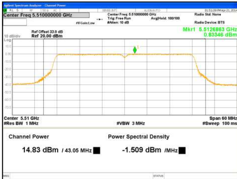
Figure 49: Maximum Conducted Output Power-5510MHz-VHT40-MCS0-Ch0
