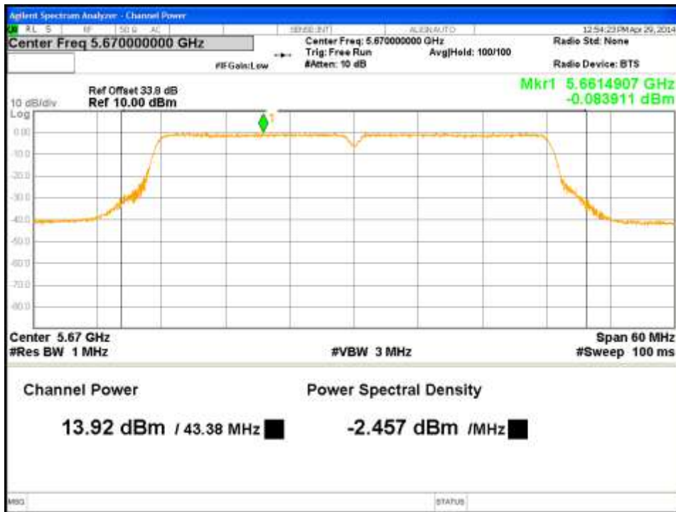
Figure 59: Maximum Conducted Output Power-5670MHz-VHT40-MCS0-Ch2
