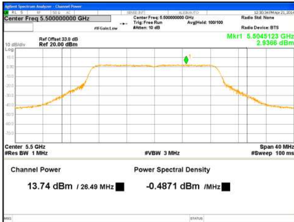
Figure 38: Maximum Conducted Output Power-5500MHz-VHT20-MCS0-Ch1
