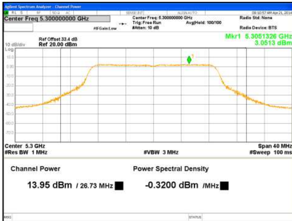
Figure 19: Maximum Conducted Output Power-5300MHz-HT20-MCS0-Ch2
