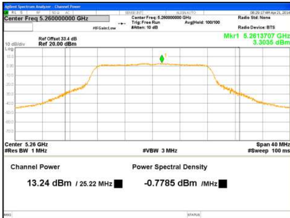
Figure 4: Maximum Conducted Output Power-5260MHz-11a-6Mbps-Ch3
