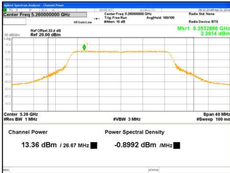
Figure 35: Maximum Conducted Output Power-5260MHz-VHT20-MCS0-Ch2
