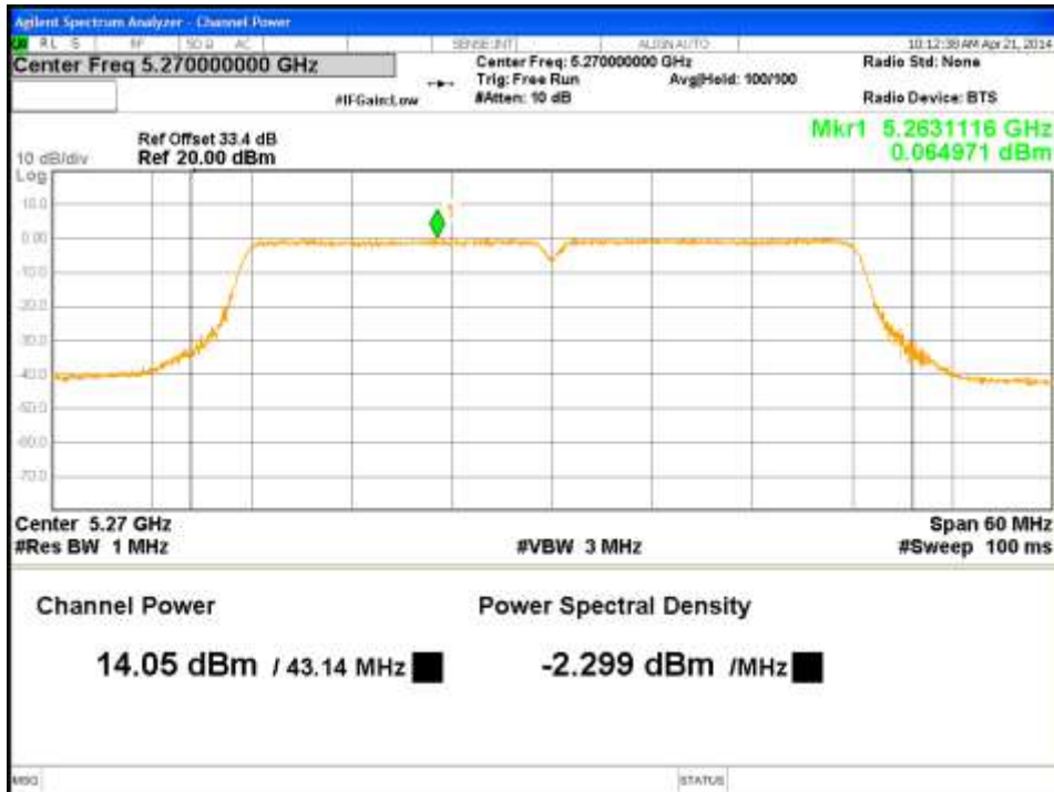
Figure 46: Maximum Conducted Output Power-5270MHz-VHT40-MCS0-Ch1
