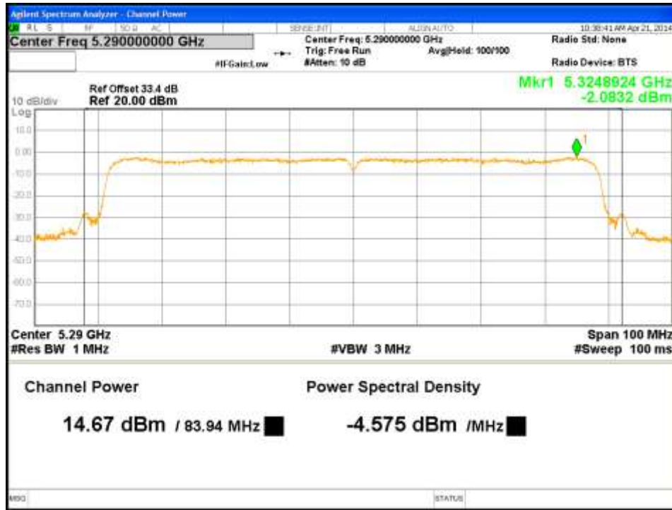
Figure 55: Maximum Conducted Output Power-5290MHz-VHT80-MCS0-Ch2
