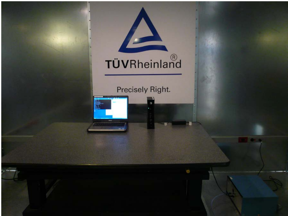
Figure 13: AC Conducted Emission Test Setup (Front View)
